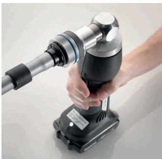
1 Expand pipe end
